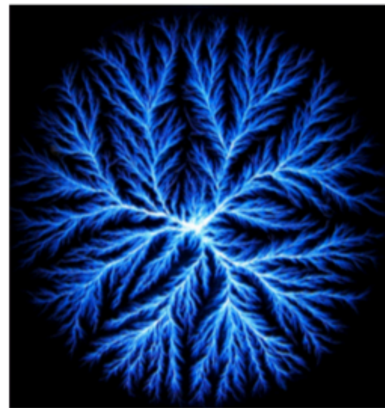
Lichtenberg "lightning", formed by rapidly discharging electrons in lucite. Scale = 10 cm = 10^{-1} m.
