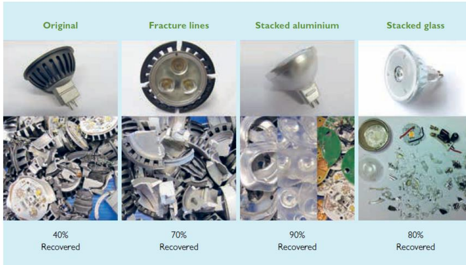
Figure 5. A LED spot light (top left) and three redesigns employing different materials and connections to improve the recycling result. The images at the bottom show typical fragments resulting from a shredding test. Recovered fractions are given in weight-%.
